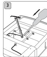
Unscrew brass links and wires.
